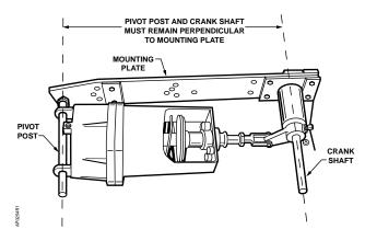
Figure 4. Perpendicular Mounting.
