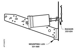
Figure 7. No. 4 Actuator Frame Mounting, Normally Closed Damper.
