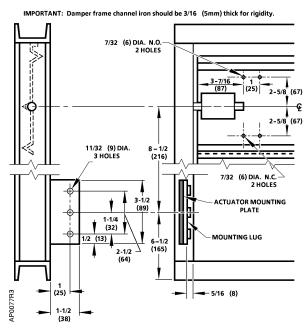
Figure 6. Frame Mounting Dimensions. Dimensions in Inches (Millimeters).
